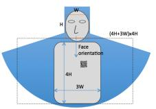
Figure 4. Search area illustration in face/Tag matching. The face and fan-shaped blue areas are the likely tagappearing area. The face area and dashed rectangular are actually used to simplify the search range.
