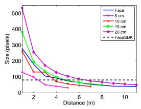
Figure 7. Size of face and tags in the photos taken at different distances.
