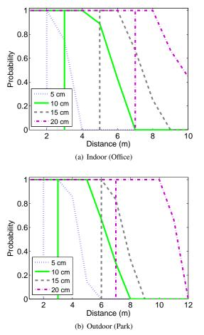
Figure 9. Detection probability different sized Tags (carrying 32Bytes) in indoor and outdoor environments.
